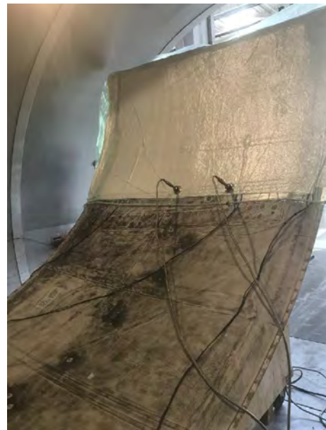
A multi zones blanket to cover the upper surface of right/left upper cowling area
