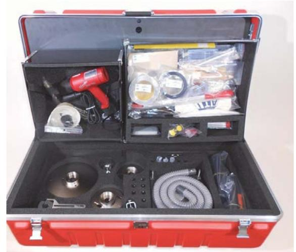
Figure 1: Complete Mobile Repair Workshop
